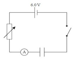
(a) When the switch is closed there is a maximum current, which decreases to zero over a period of time as the capacitor charges. Explain why.
